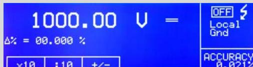
Presence of dangerous voltage over 100 V at the output terminals is always indicated by „Dangerous voltage“ sign. Calibrator indicates dangerous voltage by beeping.
